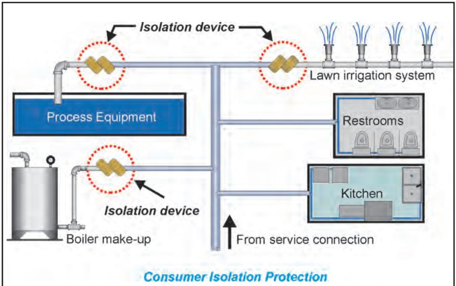
Although your plumbing system may have been constructed with great care in the past, changes in technology and safety concerns may have created the need for additional protection for your system with special backflow prevention assemblies. The City of Arvada's Building Inspection Division can assist you with isolating and protecting plumbing systems within your building.
