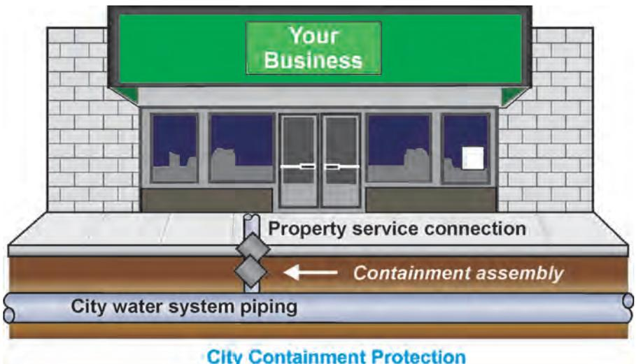
The type of backflow prevention assembly needed will depend on how the water is used within your plumbing system. Generally, water consumers will use water in one of these three applications.
